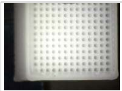
Cubic PCL scaffold structure:
