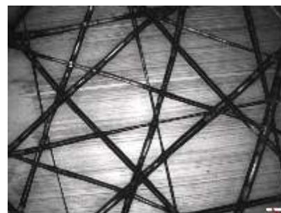
Bottom layer with 20 micron strands, top layer with 100 micron strands.
