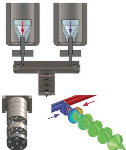
Schematic drawing of the ISG cascading mixer ("interfacial surface generator", top), enlarged view of the mixer (bottom left) and finite element simulation of the mixing process (bottom right). A stack of four to five modules is needed for complete mixing.
