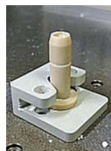
Small vial filled with 3 M KCl for pH electrode storage on the work plate
