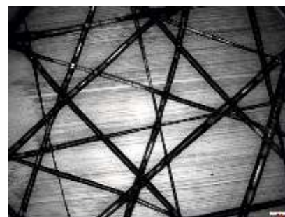
Bottom layer with 20 μm strands, top layer with 100 μm strands
