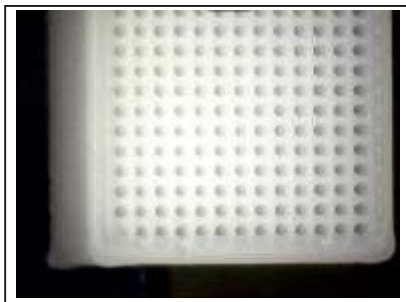
Cubic PCL scaffold structure: Edge length: 10 mm Layer height: 50 µm Number of layers: 200 Nozzle diameter: 250 µm
