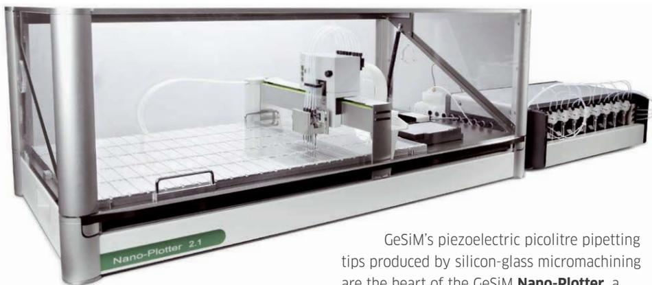
GeSiM's piezoelectric picolitre pipetting tips produced by silicon-glass micromachining are the heart of the GeSiM **Nano-Plotter**, a platform with up to 16 of these non-contact dispensers for spotting microarrays and
