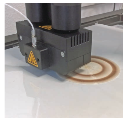
Gradient mixer in a BS5.1 dispensing concentric gradients of 0...20% zirconium phosphate + gentamicin antibiotic in PEOT/PBT
