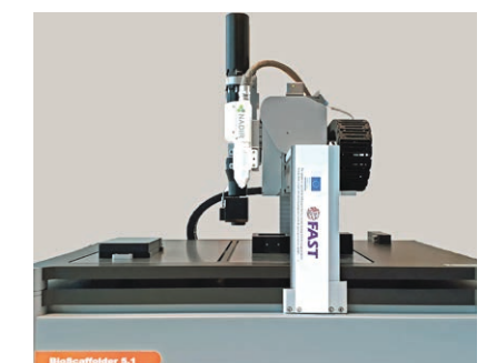
Nadir plasma jet mounted on a GeSiM BioScaffolder BS5.1. The high-temperature gradient mixer is in the back.
