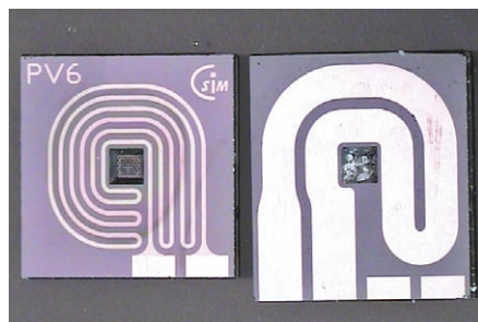
HGV PV6 actuator chamber, with platinum heater and temperature sensor structures, filled with hydrogel particles, before assembly
