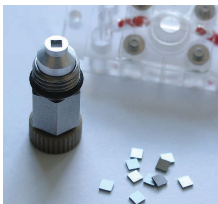
A040-083, -107 The sample carrier can bring opaque objects (up to 2.5x2.5 mm 2 ) into the flow channel; the sample must be illuminated from the objective side. The specimen can be rotated by 360°. Picture left, principle; centre, sample carrier outside channel with silicon samples; right: sample carrier screwed into its special 22x22 MicCell PC body. Please inquire for more information or other configurations.
