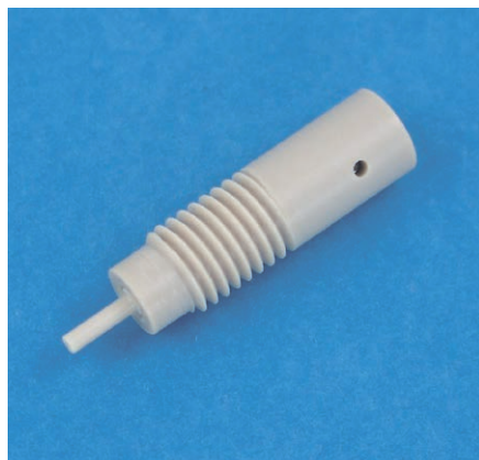
A040-091 Channel spacer, 1.6 mm diameter, in UNF1/4-28 fitting, with a spring-loaded tip. Creates a hole in the PDMS layer during gel casting.
