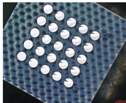
PDMS stamp, bottom view. This disposable print tool is made at your lab bench.
