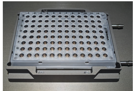
A070-351 Microtitre plate with 96 round, V-shaped wells in the adapter plate
