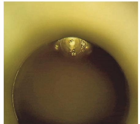
Single needle viewed from the top. In the lateral groove you can see tiny (8 µm) beads that were entrapped after fluid deposition by a piezo pipette.
