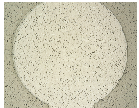
Foil-based microfluidics: microscopic image of an Oxyphen membrane with defined pores (speckles) on an adhesive foil with round hole and channel
