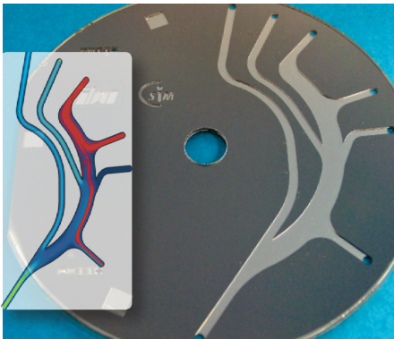
Silicon-glass channel system for magnetic separation of blood immune cells (inset: flow simulation). Project funded by BMBF, Germany.
