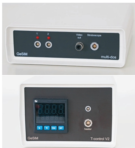
Top, multi-dos 2 for two pipettes and a stroboscope (A020-301+303); bottom, temperature control unit (A020-061) for a heatable dispenser
