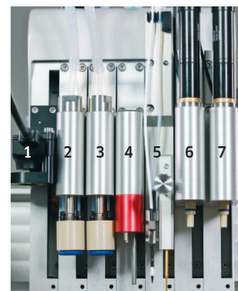
Pipetting head (example) with (1) camera, (2+3) gripper/3-lumen pipette, (4) FlipTube opener, (5) piezo tip+Z-sensor, (6+7) nozzles for needles and tips
