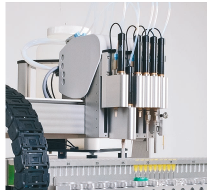
BSyS print head with nozzles for plastic tips and capillary dispensers for the production of collagen gel plugs
