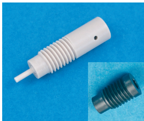
A040-091 Channel spacer in UNF ¼"-28 fitting, with spring-loaded tip (1.6 mm). Creates a hole in the PDMS layer during gel casting. Inset: A040-092, stopper fitting, UNF ¼"-28.
