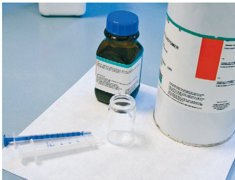
A040-514, -516, 517, -664 Large and small syringes and mixing glass for PDMS preparation, PDMS base and curing agent, syringes
