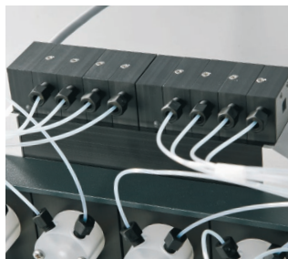
Flow sensors (8-fold on a diluter box) for droplet volume measurement
