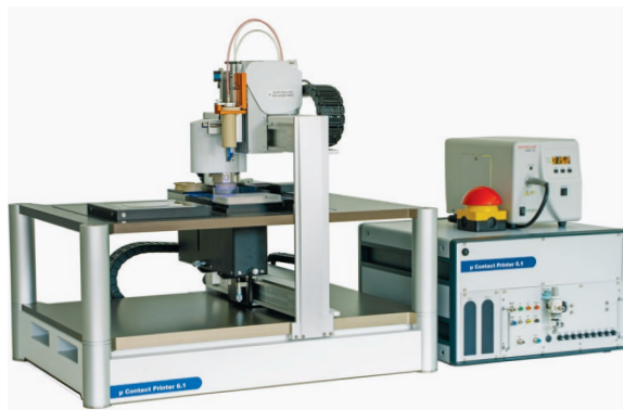
Two-level μCP6.1 with fast linear XY-motors. The lower Y-axis contains a UV collimator for precise and homogeneous irradiation especially for UV-NIL (see back page), the upper one the stamping unit. The flexible design allows easy reconfiguration.
