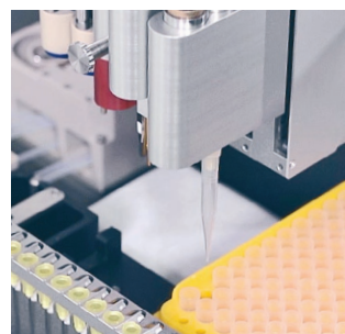
Plasma pen (Relyon) for sterilization and surface modification
