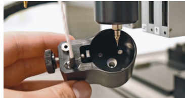
Left: Peltier-cooled cartridge holder (min. temperature 4 °C). Top: heatable cartridge holder for up to 190 °C, with tip heater and polished metal tip.
