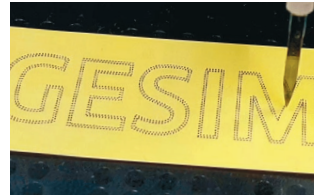
Non-contact piezo (ink-jet) printing onto water-sensitive paper. A useful alternative are solenoid valve dispensers for droplet volumes > 30 nL.
