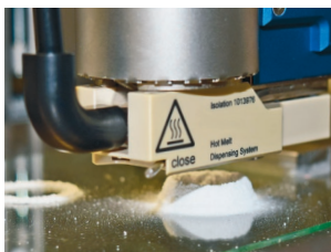
Heatable piezo valve dispenser (VERMES) printing thermoplastic
