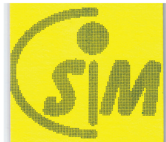
Print example: GeSIM logo on water-sensitive paper; width of the paper: 26 mm.
